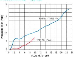
Tests conducted with units in vertical position (lead wires up) wit
