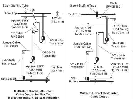
(See Fig. 8) Fig. 1 Typical Installation Arrangements of Gems 36000 Series Transmitters in the Tank
