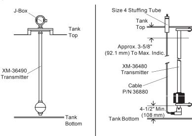
Single Unit, Bracket-Mounted, Cable Output for Max. Top Level Indication
