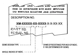
Fig 17 **Explanation of Description Number** Marked on I.D. Tag Attached to Transmitter Unit
