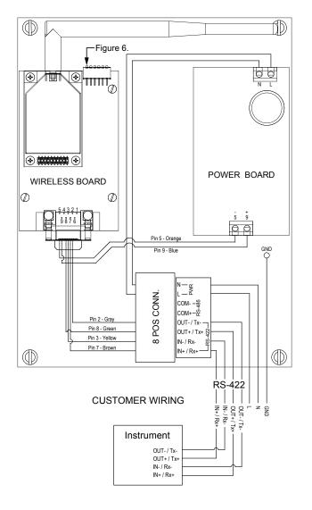
Figure 3: Wiring Diagram RS-485 (MODBUS)
