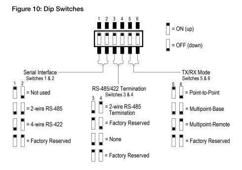
NOTE: Point to point is used when one radio is talking to one radio only; multi-point is used when there are multiple remotes and/or bases.
