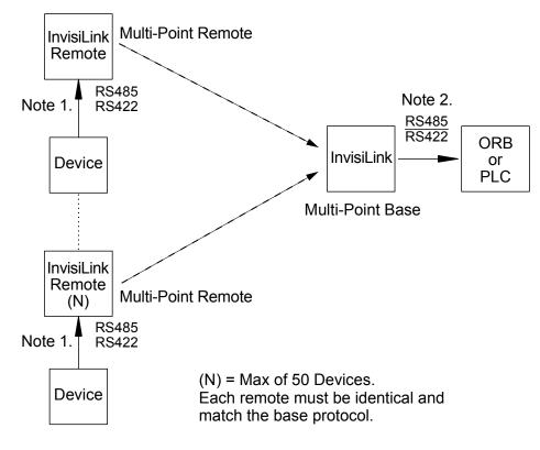
To set multi-point units, see figure 10 for dip switch settings.
