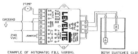
WHEN LEVEL DROPS BELOW 'A' PUMP TURNS ON. WHEN LEVEL RISES ABOVE 'B' PUMP TURNS OFF.
