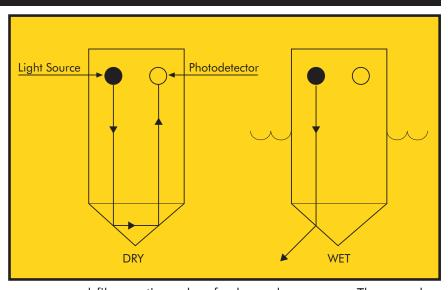
probes are designed for general purpose areas and fiber optic probes for hazardous areas. These probes are used in conjunction with a universal controller, which can be used for level alarms or pump control. The universal controller has adjustable time delay and field selectable "fail-safe" settings.
