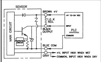
Note: Common wire (gray) must be connected to common (-) or V+(+) supply of power supply.
